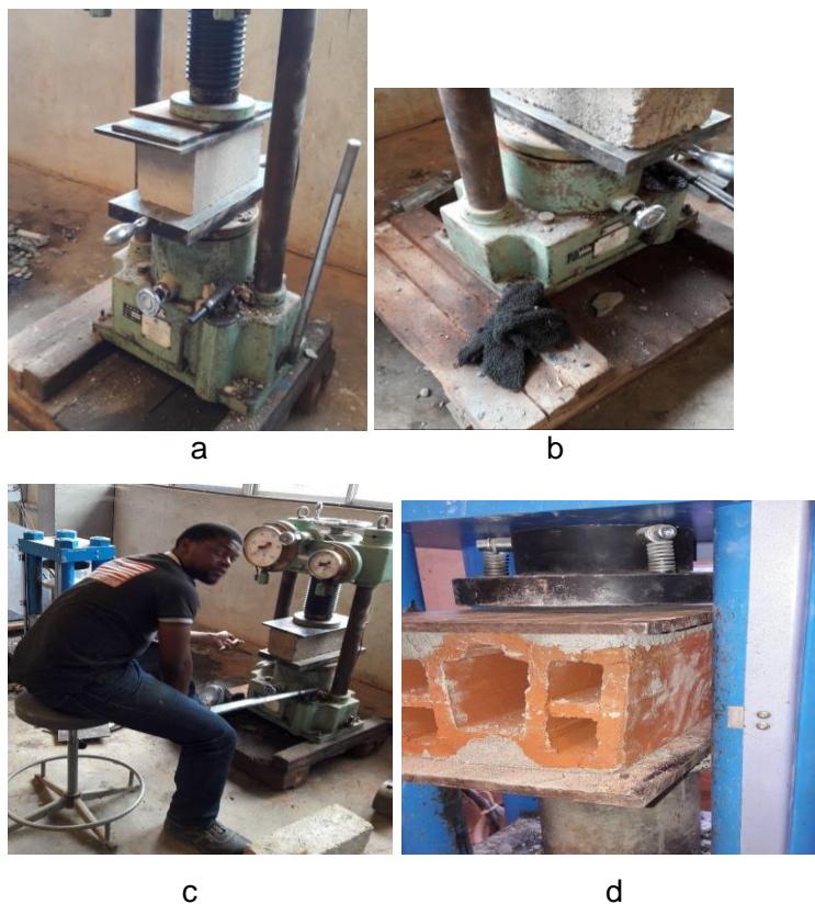
Figure 4. Compressive strength testing in a universal testing machine: (a) silicate limestone brick; (b) concrete block; (c) natural stone; and (d) clay brick.
