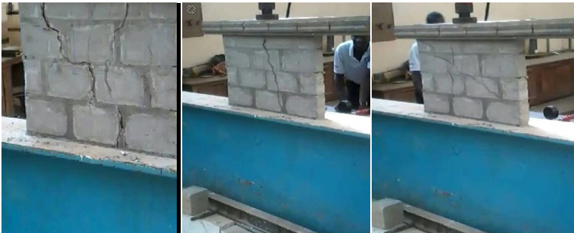
Figure 8. Crack patterns of failed wallets.
