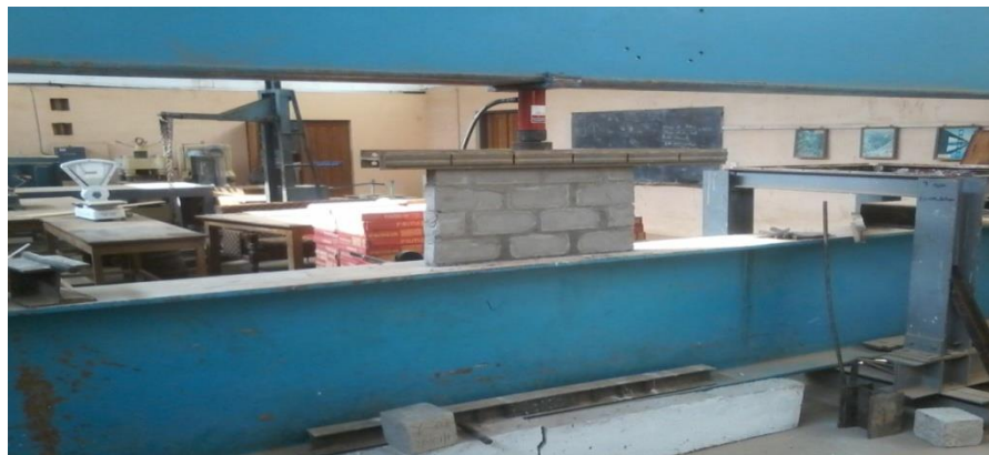
Figure 3. Test Set-up for masonry wallets compressive strength.
